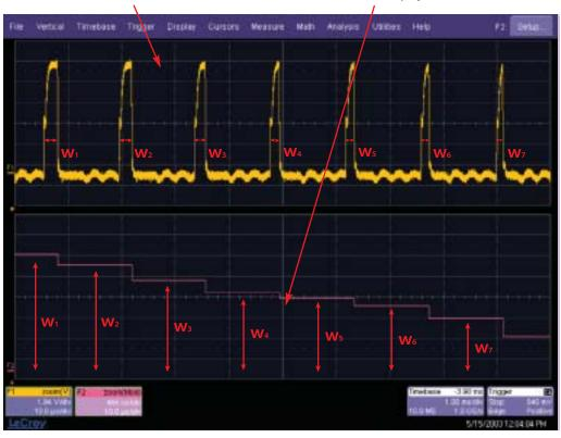
**Modulation Analysis** functions produce a time domain display, which represents the modulated parameter in a time-vs. parameter value graphical plot. They are convenient tools for intuitively viewing the time domain response of the entire control loop, including any time constants added by the pulse width modulator. Modulation Analysis can be performed for duty cycle, period, frequency, and pulse width.
